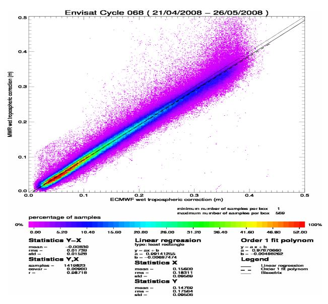
The radiometer-model mean difference is 0.8 cm. A drift on the Envisat 23.8GHz brightness temperature has been detected and has to be monitored on the long term. Note that the neural algorithm is now implemented on Envisat.
