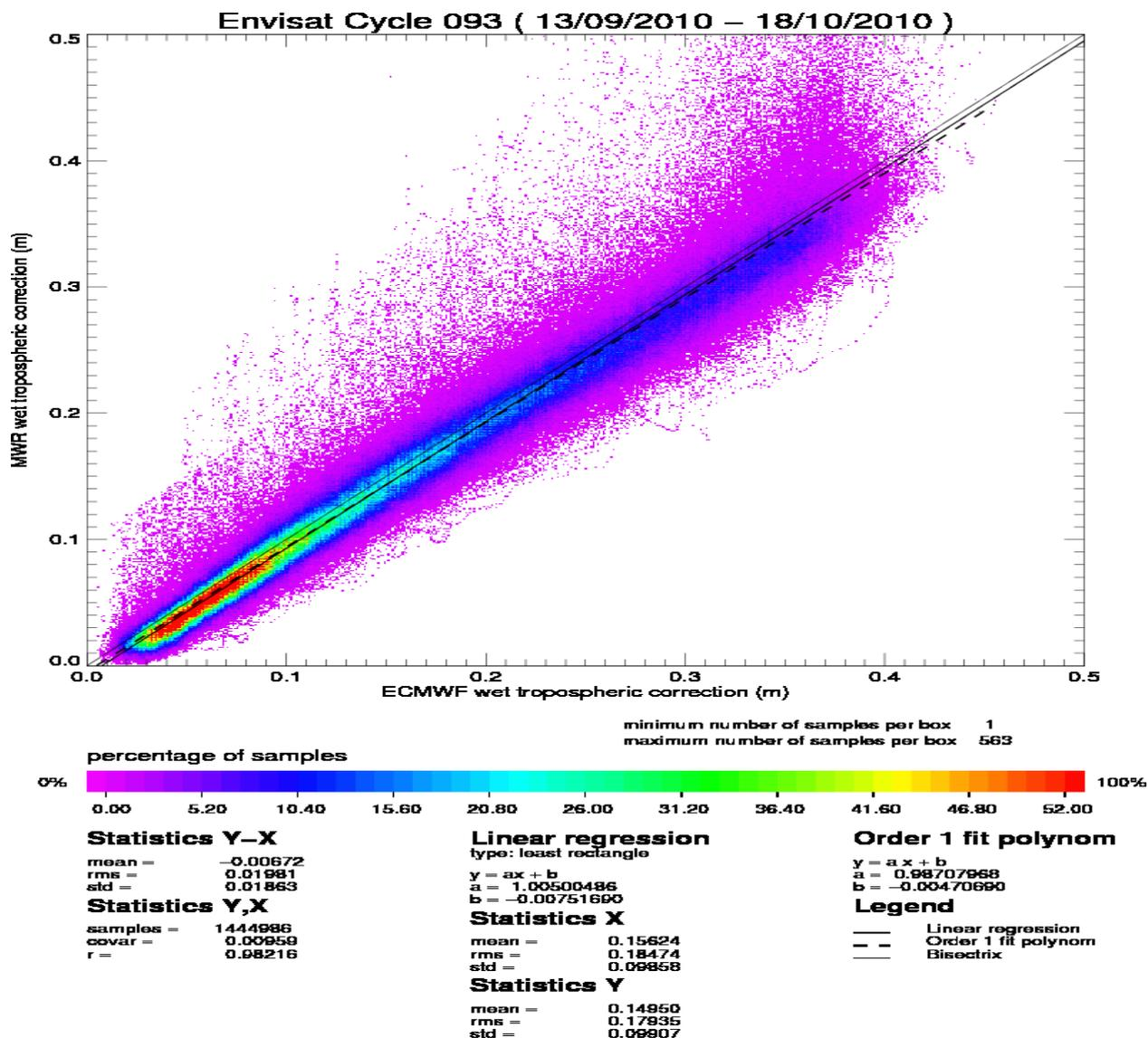
The radiometer-model mean difference is 0.7 cm. A drift on the Envisat 23.8GHz brightness temperature has been detected and has to be monitored on the long term. Note that the neural algorithm is now implemented on Envisat.
