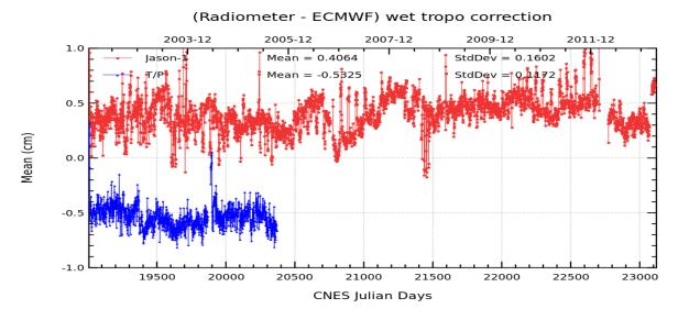
Daily monitoring of the radiometer minus model wet troposphere difference increases of about 1mm on 2013-04-17 (related to yaw ramp) and then decreases until the end of the cycle (-1mm) (see figure below). The increase observed in IGDR is significantly reduced thanks to the new radiometer calibration file.
